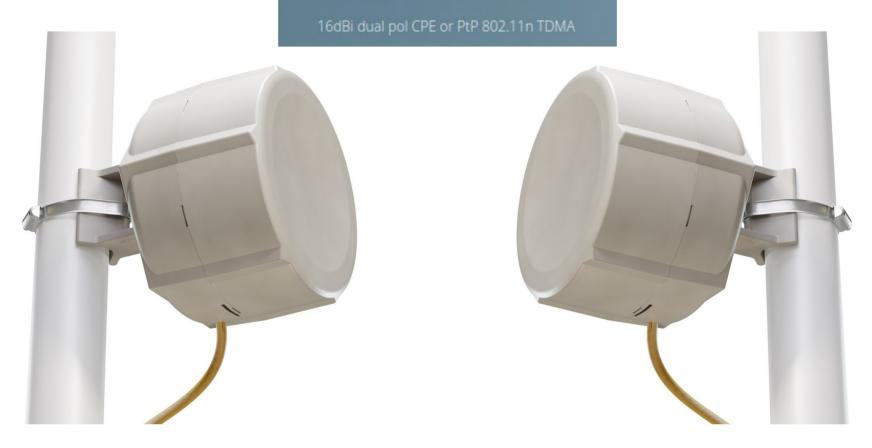
Our integrated outdoor unit for Point-to-point, or as a CPE device for point-to-multipoint.
